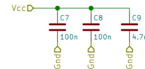
Place decoupling capacitors as close to power inputs on microcontroller as possible.
