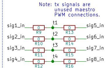
Solder bridges can be used to short over different signals to different inputs on the isolators. This is for potential faults within the maestro.
