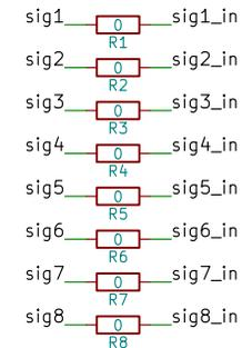
Solder bridge connections must be shorted to mux inputs for the input signals to be transmitted.
