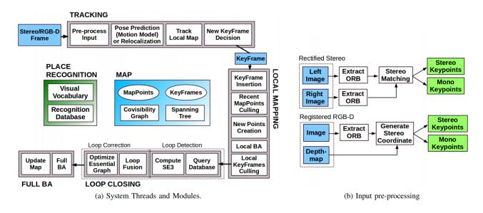
ORB-SLAM2 is a feature based algorithm that takes keyframes from video output and extracts keypoints or features (such as corners), and uses them to establish location of the sub and its surroundings.
