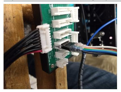
4. Connect the wire charging cable (the one without the plastic wrapping) into the power connector of the battery box. Connect the red connector to the cable with the red zip tie and the black connector to the black wire.
