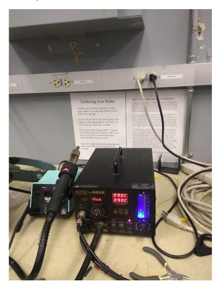
Heat up the heat gun to 90 degrees Celsius. Shrink all of the small heat shrink at the same time, over the solder joints (not pictured).
