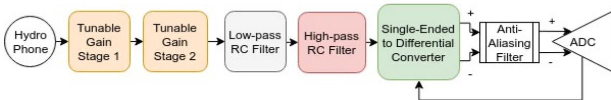
The analog signal goes through a five-stage amplification and filtering process. First, the signal is sent through two gain stages, each of which apply an adjustable gain to the signal. After the signal is gained into a reasonable voltage range, it is passed through a low-pass filter and then a high-pass filter to result in a bandpass filter of the signal.
