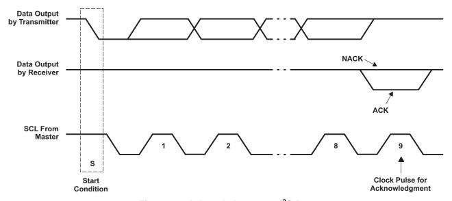
Figure 11. Acknowledgment on I<sup>2</sup>C Bus
