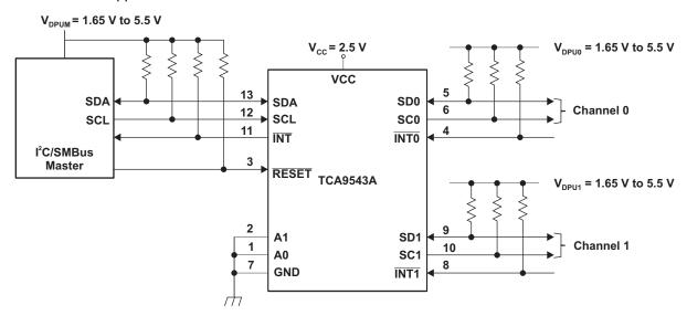
Figure 16. Typical Application Schematic
