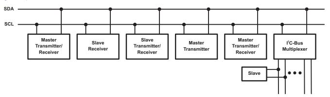
Figure 10. System Configuration
