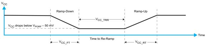
Figure 20. V<sub>CC</sub> is Lowered Below the POR Threshold, Then Ramped Back Up to V<sub>CC</sub>
