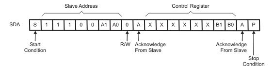
Figure 12. Write Control Register
