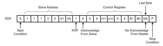
Figure 13. Read Control Register
