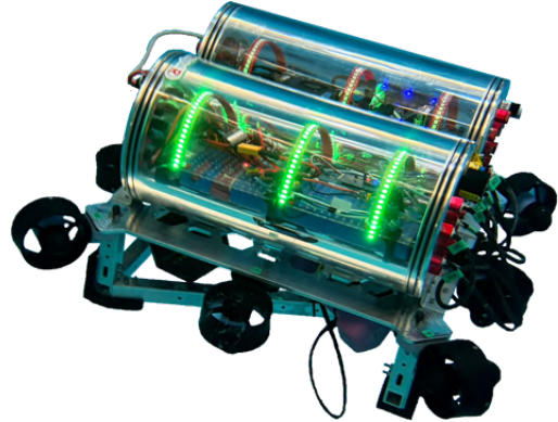
Fig. 1. Guppy: Palouse RoboSub’s Autonomous Underwater Vehicle.
