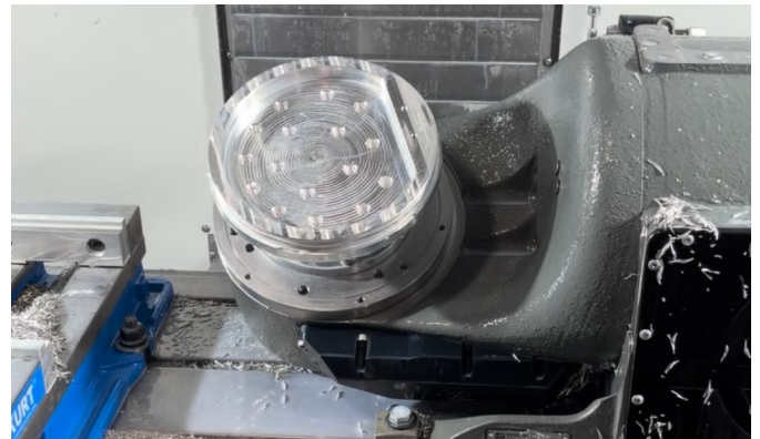
Fig. 2. Haas VF2SS with a TRT210 trunnion and a Guppy endcap.
