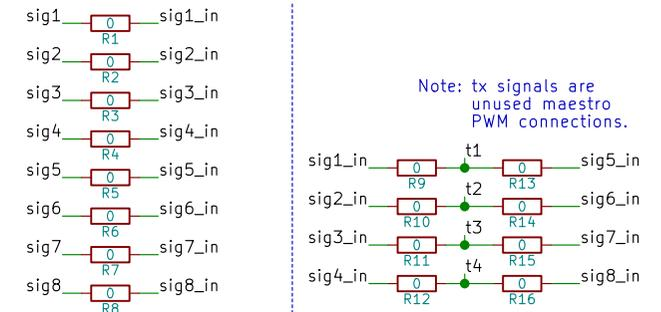
Solder bridge connections must be shorted to mux inputs for the input signals to be transmitted.
