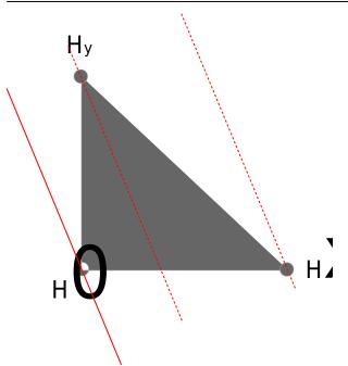
Because the wave emanating from the pinger hit  $H_x$  before it hit  $H_0$ , we know that  $H_x$  must be closer to the pinger than  $H_0$ . In fact,  $H_x$  must be exactly  $d_x = c_s(t_0 - t_x)$  meters closer to the pinger than  $H_0$ . Likewise,  $H_y$  is  $d_y = c_s(t_0 - t_y)$  meters closer to the pinger
