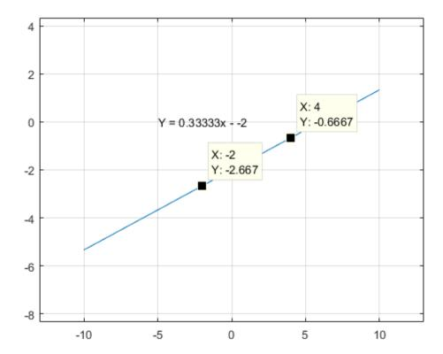
Now let's try fitting a line to an over-determined set of points. Below 20 points have been randomly generated. The x components were are uniformly random samples across domain [-10, 10]. The corresponding y components were first calculated directly using the true line equation  $y = -\frac{1}{3}x - 2$ , and subsequently adding samples from a Gaussian random distribution with standard deviation  $\sin x = 0.5$ .
