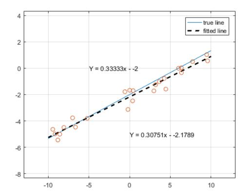
We've just estimated our state based off of noisy measurements in an optimal fashion. At it's core, line-fitting like this is all that the Kalman Filter is doing. These next sections we will continuously build upon this basic function until we have something resembling the Kalman Filter.
