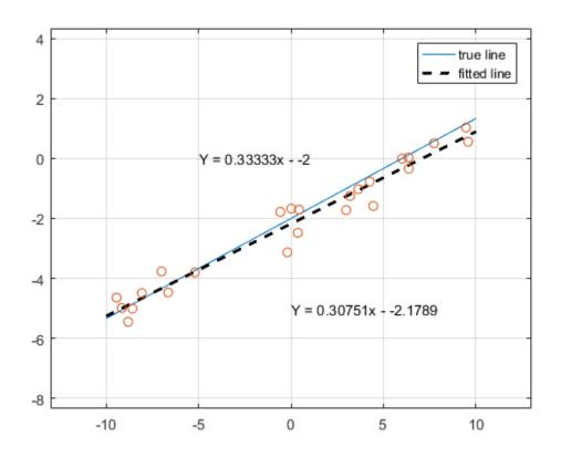
We've just *estimated* our *state* based off of *noisy* measurements in an optimal fashion. At it's core, line-fitting like this is all that the Kalman Filter is doing. These next sections we will continuously build upon this basic function until we have something resembling the Kalman Filter.
