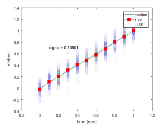
We see that at each point in time, we take many measurements, and estimate a position that is close to our true position. If we did this 1000 times, we can see how accurate we are at tracking our system
