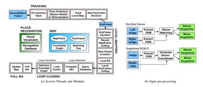
ORB-SLAM2 is a feature based algorithm that takes keyframes from video output and extracts keypoints or features (such as corners), and uses them to establish location of the sub and its surroundings.
