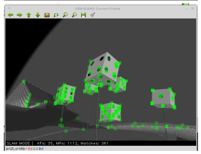
The view of a single keyframe with detected map points.
