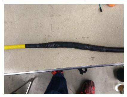
Wrap the splice in electrical tape. Start with a few wraps on one side, have the tape overlap half of itself as it winds up the splice and then end with a few wraps on the opposite side. Make sure the heat shrink is tight.
