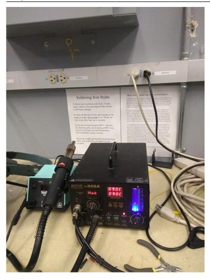
Heat up the heat gun to 90 degrees Celsius. Shrink all of the small heat shrink at the same time, over the solder joints (not pictured).
