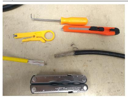
Remove the outer jackets of both cables
