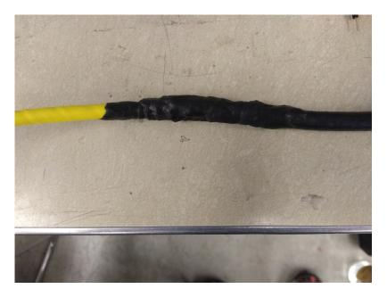
Cover the entire splice in 3M window weld. Make sure that there are no gaps. Try to make it thin enough that the larger heat shrink can fit over it after it is covered in electrical tape.
