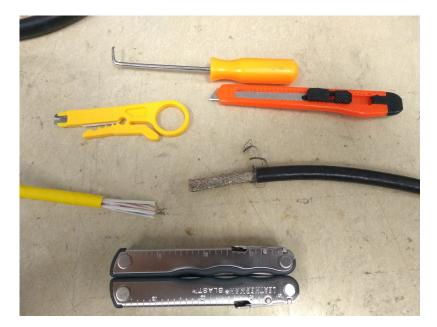
Remove the outer jackets of both cables
