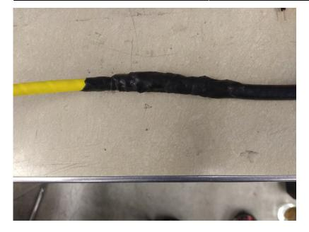
Cover the entire splice in 3M window weld. Make sure that there are no gaps. Try to make it thin enough that the larger heat shrink can fit over it after it is covered in electrical tape.
