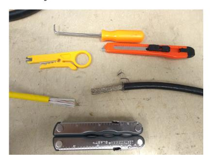
Remove the outer jackets of both cables
