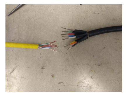
Make sure there is enough bare metal that there is enough length for each bare wire to wrap around each other. Also make sure the small heat shrink is long enough to cover the solder joint.
