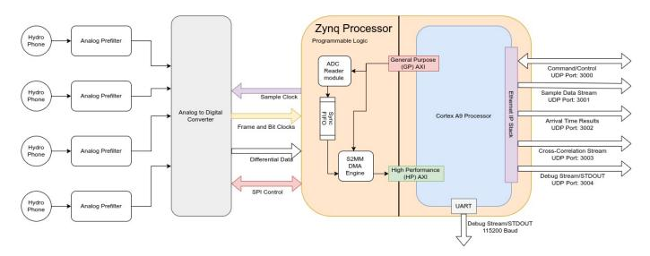
The hydrophones have small piezo sensors that output very small voltages as sound hits them. To be able to read them, the hydrophone signals are filtered with a 1st order bandpass and then are gained by approximately 40-60dB. After the signals are amplified, they are then passed to the ADC for
