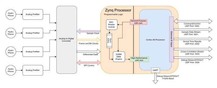
The hydrophones have small piezo sensors that output very small voltages as sound hits them. To be able to read them, the hydrophone signals are filtered with a 1st order bandpass and then are gained by approximately 40-60dB. After the signals are amplified, they are then passed to the ADC for
