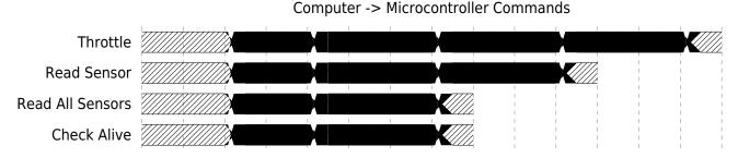
The first two commands are the basic interface for controlling the thrusters and getting information. There is the third macro command for reading all the registers of a thruster. There is no macro command for talking to all thrusters because this would require the microcontroller to know what thrusters exist/are active on the sub, which would complicate the code. The final command is a method for checking if a thruster is alive and responding, it will return a bool true/false value.
